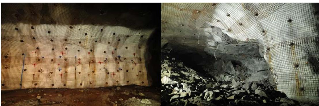
Figure 1-3 a) Panel after zero test 1, b) after zero test 3 (Photo Nordqvist, LKAB).
