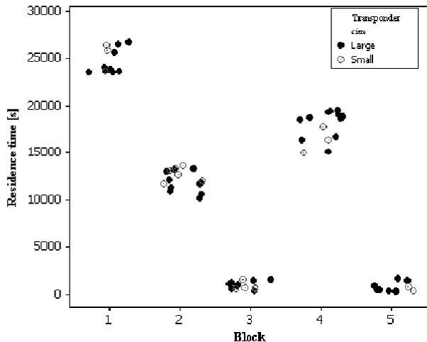
**Figure 3.** Transponder residence times for the experiment. The difference in mean residence time depends on intermittent loading of trains.
