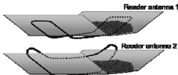
*Figure 2. The two reader-antenna shapes. The antenna of reader 1 is mounted under the conveyor and the antenna of reader 2 is mounted around it.*
